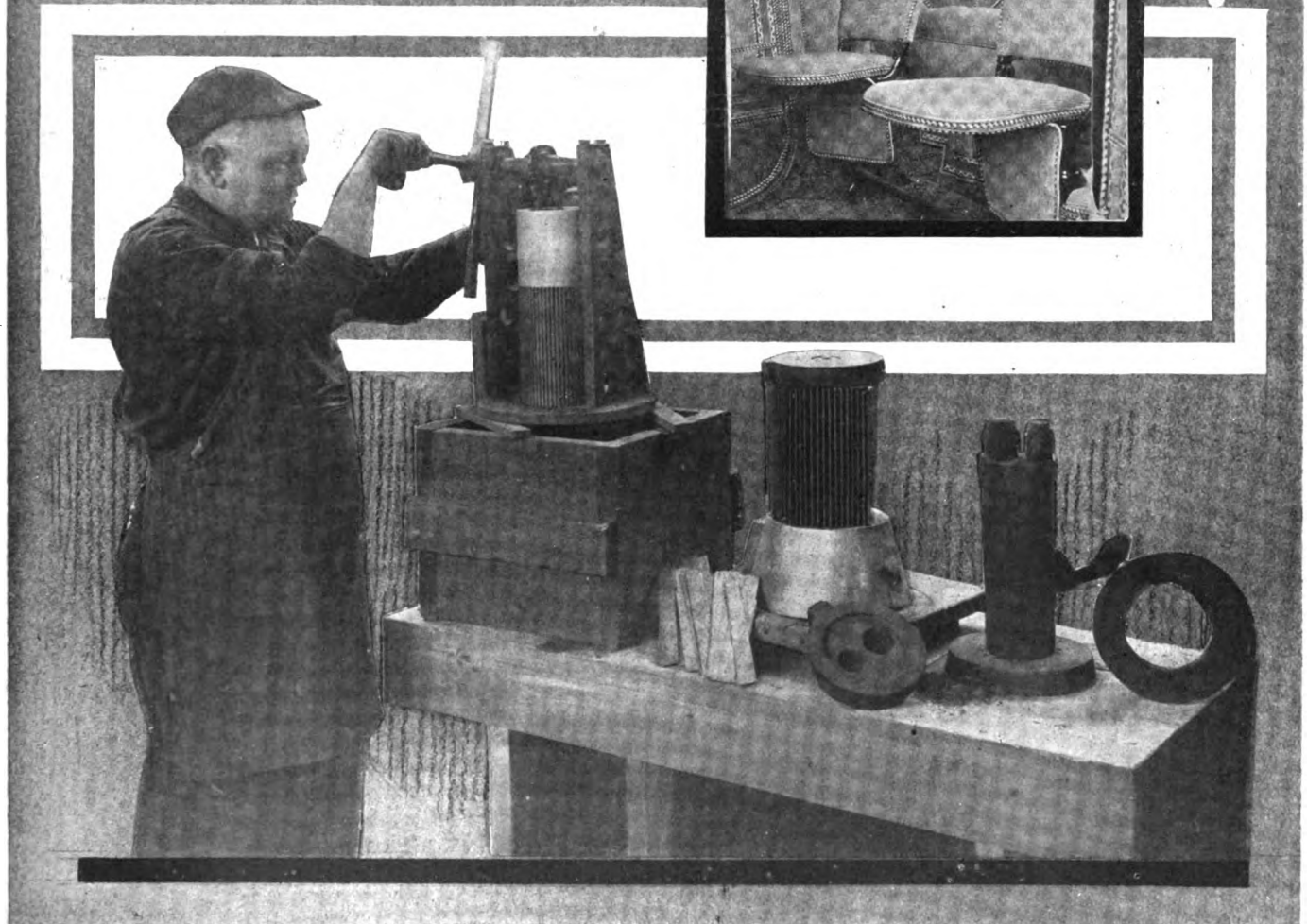
HOW THE FRANKLIN CYLINDERS ARE MANIPULATED IN THE FOUNDRY TO WELD THE VENTILATING STRIPS TO THE CASTINGS—INTERIOR VIEW OF THE THOMAS-FLYER TOWNCAR BROUGHAM
